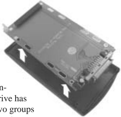
**Step 4:** Look at the hard drive connector pins and observe that the drive has two groups of such pins. These two groups are separated by a noticeable gap in the sequence of pins. The first group (Group A) has 22 contiguous 2-pin columns (which actually has one pin missing in the middle of one of its rows). The second group (Group B) has just 2 columns of pins and is located at the left end of the drive connector.
