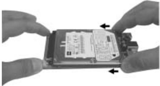
**Step 8:** Making sure that the hard drive does not fall, turn the PCB/hard drive assembly over and secure the drive to the PCB. Screw the four short metric screws provided into either the four outer screw slots or the four inner slots, depending on the drive installed.
