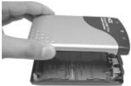
**Note:** The faceplate surrounding the Transport Pro's FireWire/USB ports is removable and may come out of its slot. If so, simply remember to put it back before replacing the enclosure's top cover later.
