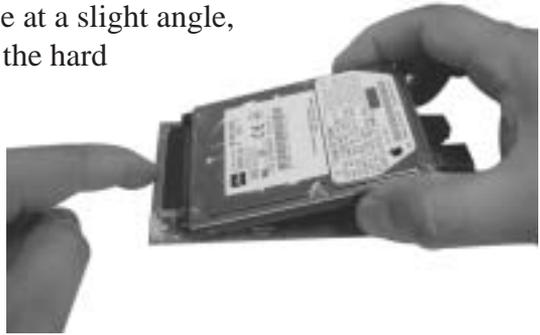
**Step 7:** Once the tips of the hard drive pins are inserted, you can lay the drive down onto the PCB. Holding the left end of the PCB with your left hand, carefully but firmly push the hard drive to the left with your right thumb and index finger to completely insert the hard drive pins into the connector.
