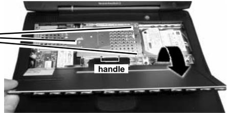
**Step 8:** Remove the heatsink by removing its three screws and pulling its handle up and out.
