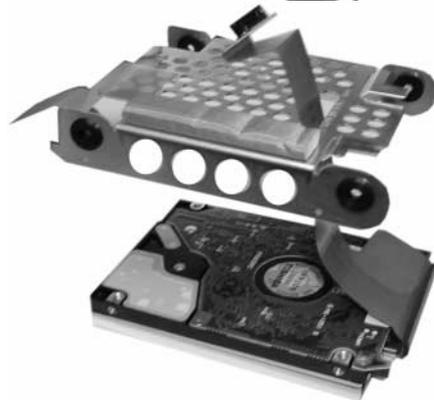
**Step 14:** Carefully remove the ribbon cable connector from the hard drive.
