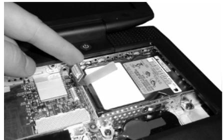
**Step 11:** Disconnect the hard drive ribbon connector from the logic board.
