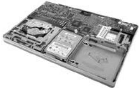
**Step 7:** Disconnect the hard drive connector from the logic board.
