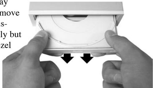
**Step 11 (c):** You can then simply slide the bezel up and remove it from the drive. Push the drive's tray back into the drive.
