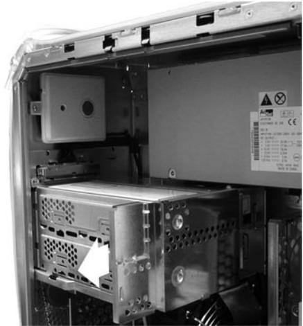
**Step 7:** Remove the power and ribbon cables from the optical drive.
